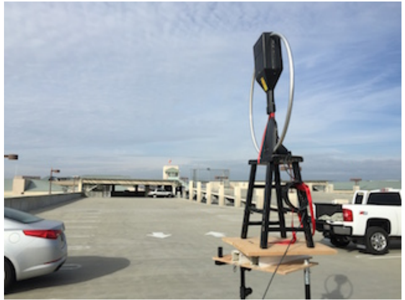
MJF Magnetic loop rotated 90 degrees from I-80 ("W-E"). Heliport, seen in background, limits antenna height.
